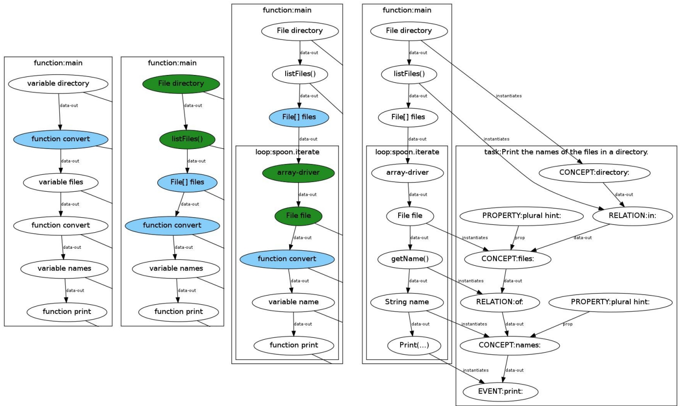
Fig. 1. Four of Macho’s candidate solutions for “Print the files in a directory”. The easiest way to understand this diagram is to start at the right, with the block labeled “Task:Print the names of the files in a directory”. This contains the skeleton program generated from the parse tree; the verb ‘print’ has become an event, the nouns ‘names’, ‘files’, and ‘directory’ have become concepts, and the prepositions ‘in’ and ‘of’ have become relations. The box immediately to the left (second from the right) is the best solution. Each event has been mapped to a function and each noun to a variable. The three boxes on the left show intermediate solutions, starting with an empty program that matches the structure of the skeleton. All of them include a copy of the skeleton program (you can see the lines going off to the right for each node) that has been removed to save space. The second candidate is generated from the first one by the database pattern selecting the java.io.File.listFiles() function for the directory to files conversion, and the third candidate is generated from the second by Macho trying a for loop over the resulting array. For more details see section II-G.
